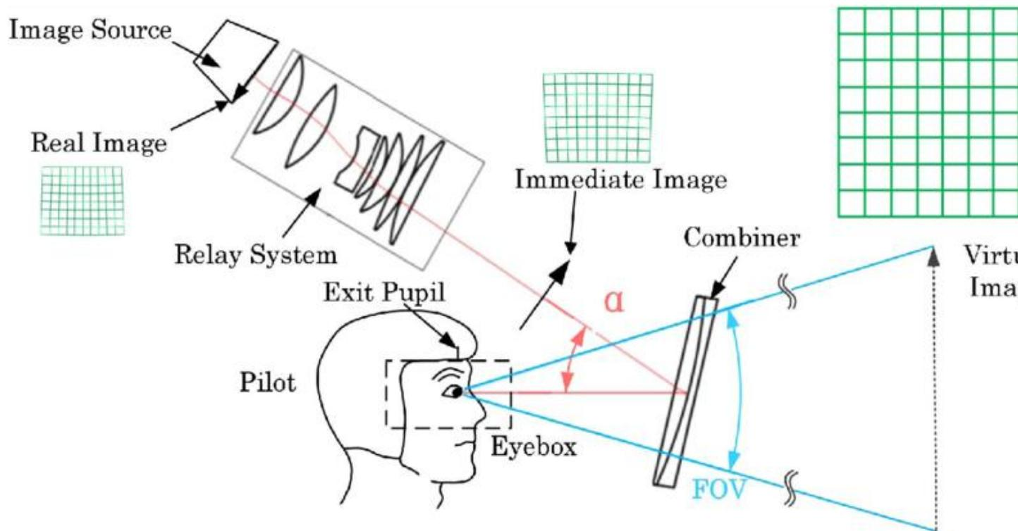
**fig: Schematic diagram of HUD.**
