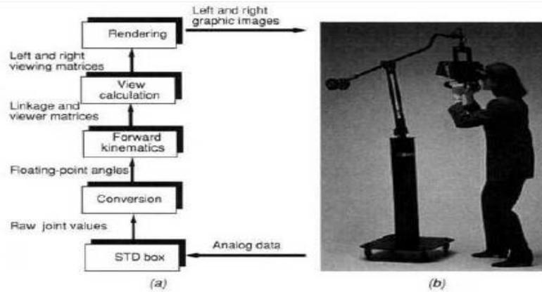
Fig. 3.8 The Boom3C floor-supported display: (a) data flow. Adapted from McDowall et al. [1990]. Reprinted by permission. (b) General appearance. Courtesy of Fakespace Labs Inc.
