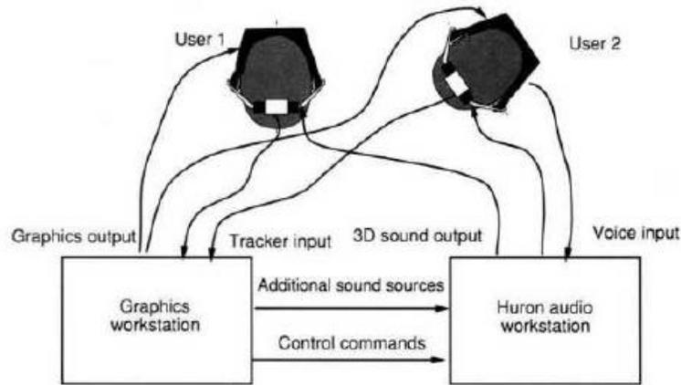
Fig. 3.24 The Huron 20 audio workstation. Adapted from Lake Technology [2002]. © Lake Technology Ltd. Reprinted by permission.
