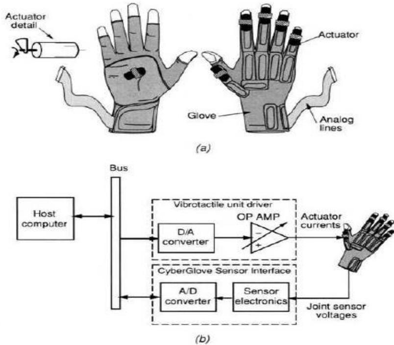
Fig. 3.28 The CyberTouch glove. Adapted from Tremblay and Yim [2000]. © 2000 Immersion Co. Reprinted by permission.
