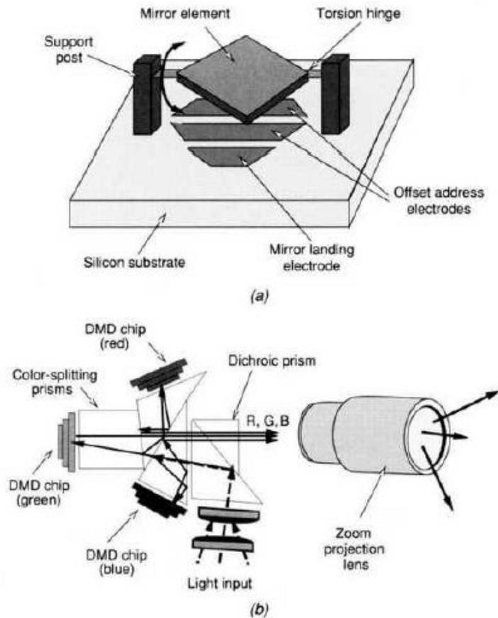
Fig. 3.15 Digital Micromirror Device (DMD) display: (a) the micromirror element. Adapted from Youse [1993]; (b) the Texas Instruments DMD-based projector. Adapted from Lubell [2000]. © 1993, 2000
