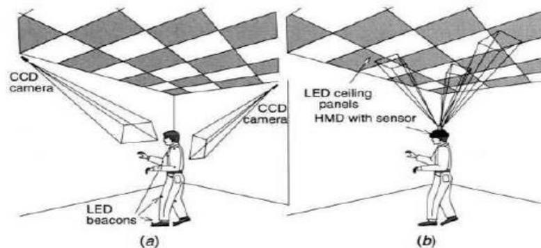
Fig. 2.16 Optical tracker arrangement: (a) outside-looking-in; (b) inside-looking-out. Adapted from Welch et al. [2001]. © 2001 Massachusetts Institute of Technology. Reprinted by permission.
