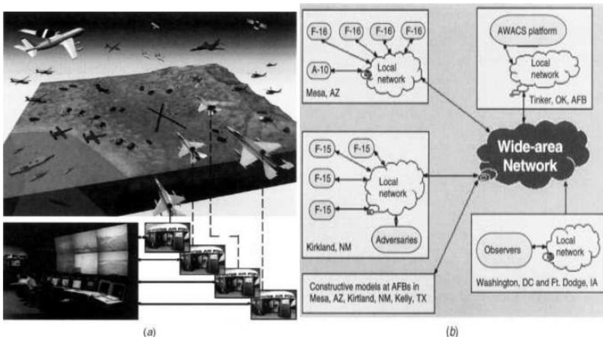
Distributed Mission Training (DMT) simulators. (a) Networked units. From Air Force Research Laboratory [2002b]. Reprinted by permission. (b) RoadRunner'98 DMT largescale exercise configuration.
