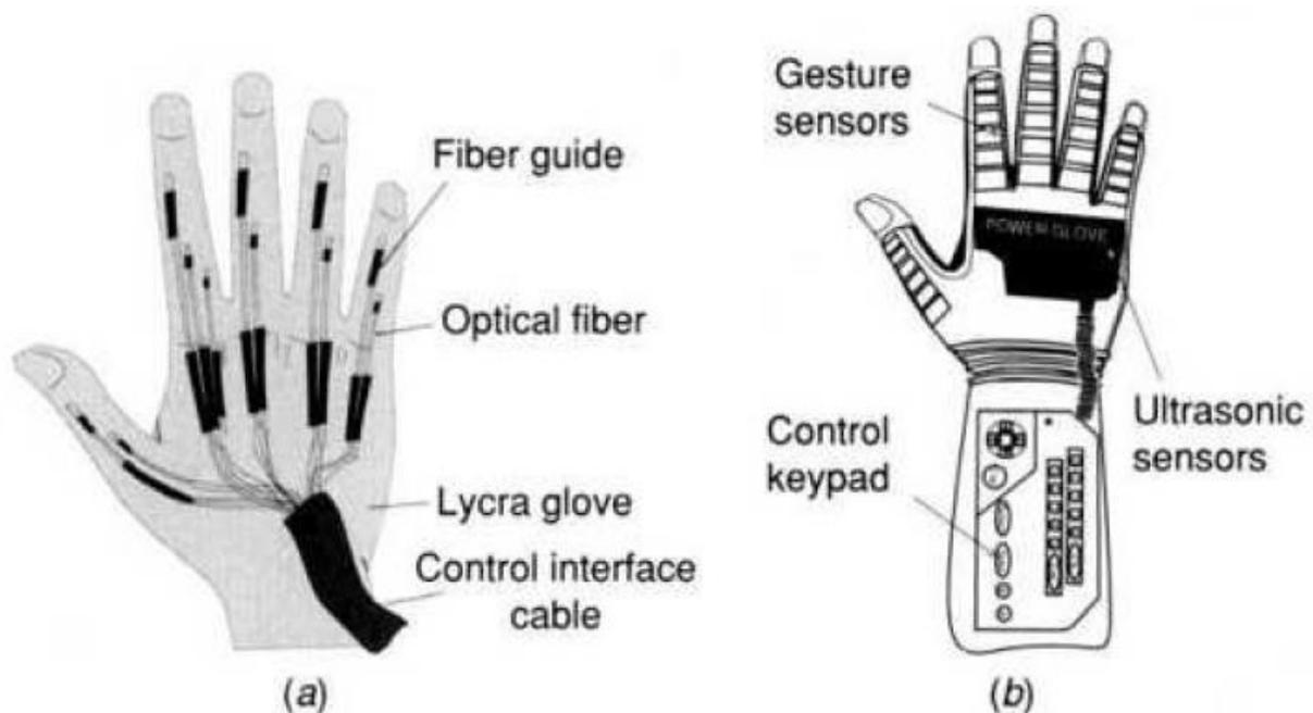
Above Fig. shows Early sensing glove technology: (a) the VPL DataGlove; (h) the PowerGlove. From Burdea [1993]. Reprinted by permission.
