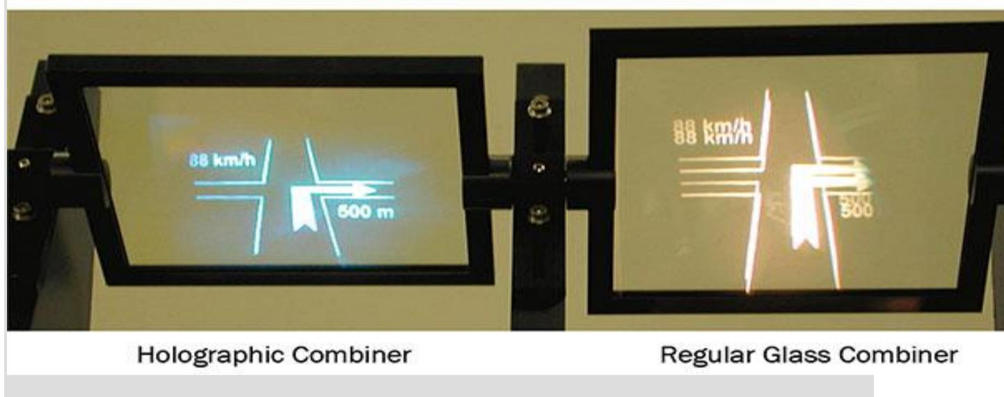
**Figure 2. A holographic combiner (left) and a regular glass combiner (right). Note the doubling of the image in the case of the simple glass combiner. Courtesy of Pierre-Alexandre Blanche.**
