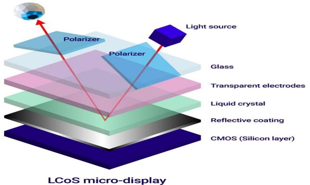
LCoS modulates light from an external source to produce the image
