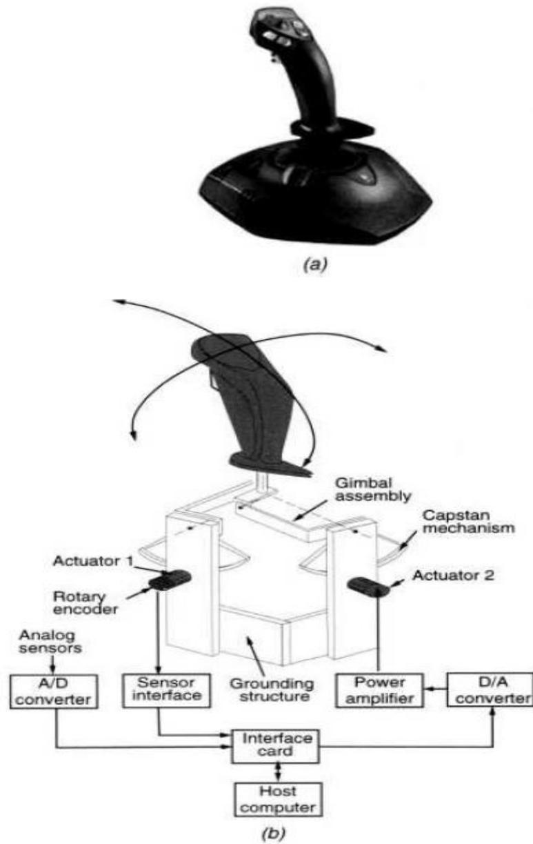
Fig. 3.30 The WingMan<sup>®</sup> Force<sup>™</sup> 3D joystick. (a) Outside appearance. From Logitech Co. [2001]. © Logitech. All rights reserved. Logitech, the Logitech logo, and other Logitech marks are owned by Logitech and maybe registered. Reprinted by permission. (b) The force feedback system. Adapted from Rosenberg [1998]. © 1998 Immersion Co. Reprinted by permission.
