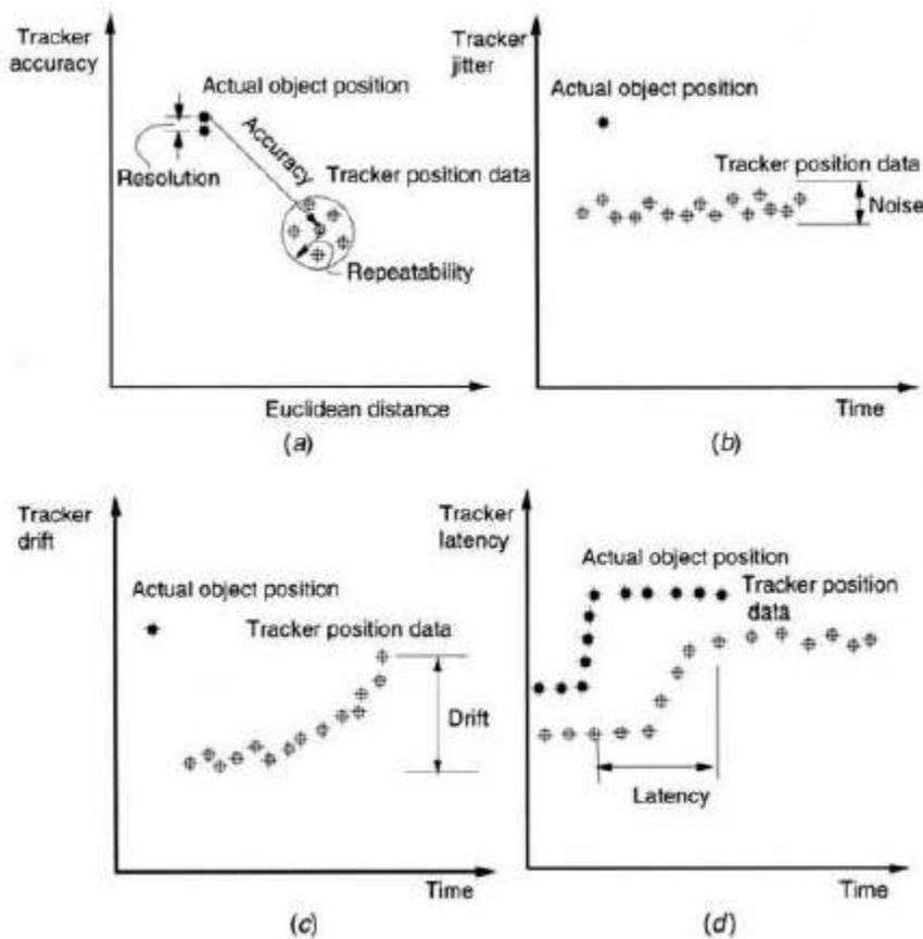
Fig: Tracker performance parameters: (a) accuracy; (b) jitter; (c) drift; (d) latency.
