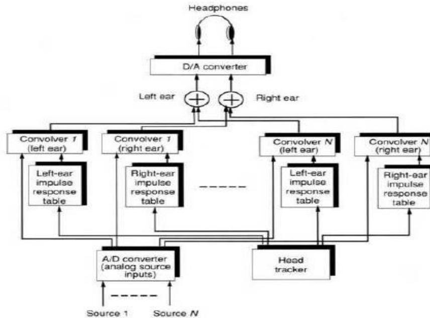
Fig. 3.23 The generic Convolvertron block diagram.
