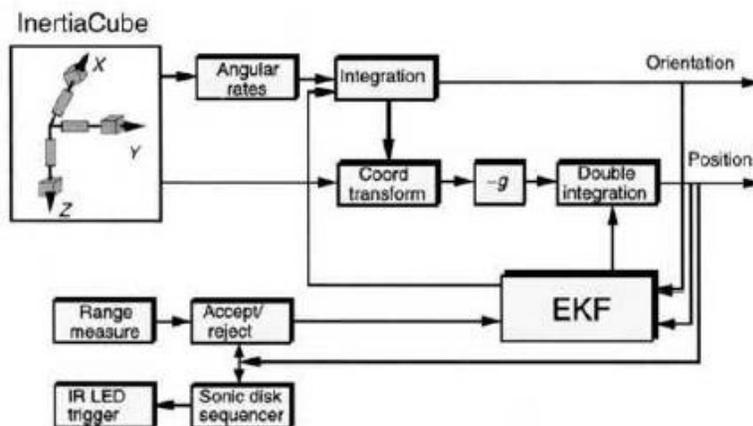
Fig. 2.20 The InterSense Inc. IS-900 software block diagram. Adapted from Foxlin et al. [1998]. © 1998 ACM Inc. Reprinted by permission.
