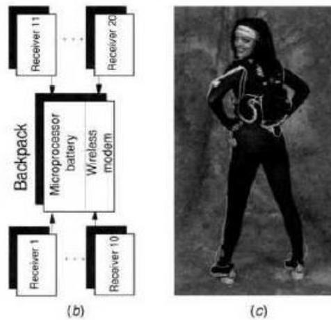
Fig. 2.12 MotionStar© wireless system: (a) block diagram; (b) back pack unit. Adapted from Ascension [2001b]; (c) User wearing the tracking suit. © Ascension Technology Co. Reprinted by permission.
