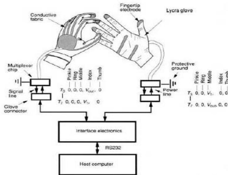
Fig. 2.26 The Pinch Glove block diagram. Adapted from McDowall et al. [2000]. Reprinted by permission of Fakespace Labs, Inc.
