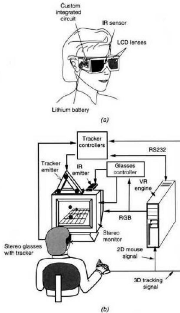
Fig. 3.12 Single CRT-based large-volume display. (a) Active stereo glasses. From Burdea [1993]. Reprinted by permission. (b) Communication diagram. From Burdea and Coiffet [1993]. © Editions
