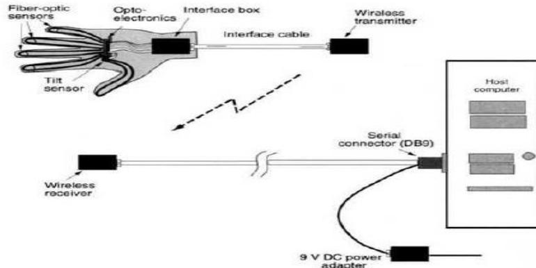
Fig. 2.27 The 5DT Data Glove 5W block diagram. Adapted from Fifth Dimension Technology Inc. [2000]. Reprinted by permission.
