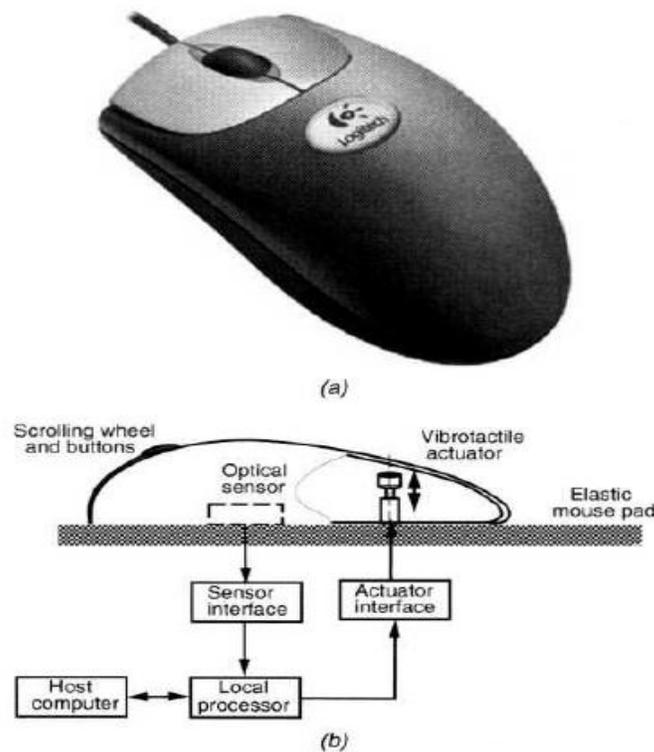
Fig. 3.27 The iFeel™ tactile feedback mouse. (a) Outside appearance. From Logitech Co. [2002]. © 2002 Logitech. All rights reserved. Logitech, the Logitech logo, and other Logitech marks are owned by Logitech and may be registered. Reprinted by permission. (b) Tactile feedback system. Adapted from Rosenberg and Martin [2001]. © 2001 Immersion Co. Reprinted by permission.
