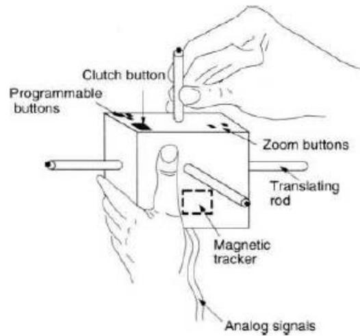
Fig. 2.21 The Cubic-Mouse. Adapted from Frohlich et al. [20001. © 2000 IEEE. Reprinted by permission.
