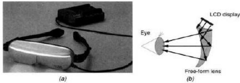
Fig. 3.4 The Olympus LCD-based Eye-Trek FMD: (a) the FMD 200; (b) optics arrangement. Adapted from Olympus Co. [2001]. Reprinted by permission.
