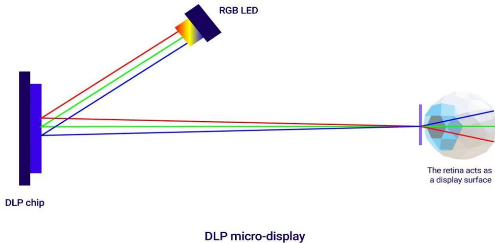
DLP Micro displays are one of the fastest display technologies in existence. Their speed of color refresh, low latency, low power consumption and extreme high resolutions (0.3 inch array diagonal enables a 1280 x 720 image) make them ideal candidates for building head-mounted displays.
