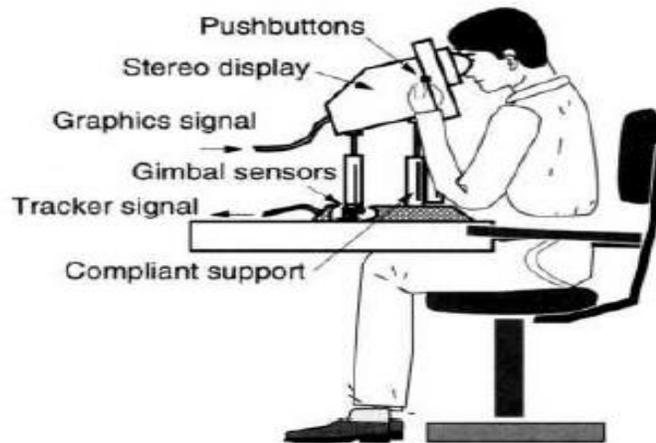
. 2.5 Mechanical tracker used in the Push 1280 stereo display. Adapted from Mead et al. |
