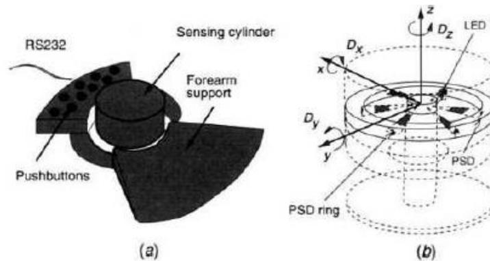
Fig. 2.22 The Magellan trackball: (a) outside configuration; (b) the sensing mechanism. Adapted from Hirzinger and Bejczy [1988]. Reprinted by permission.
