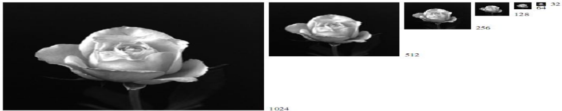
Fig.7.1. A 1024*1024, 8-bit image subsampled down to size 32*32 pixels The number of allowable gray levels was kept at 256
