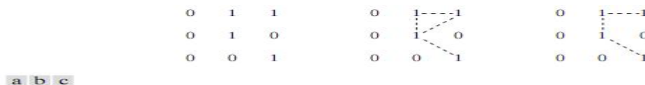
Fig.9 (a) Arrangement of pixels; (b) pixels that are 8-adjacent (shown dashed) to the center pixel; (c) m-adjacency
