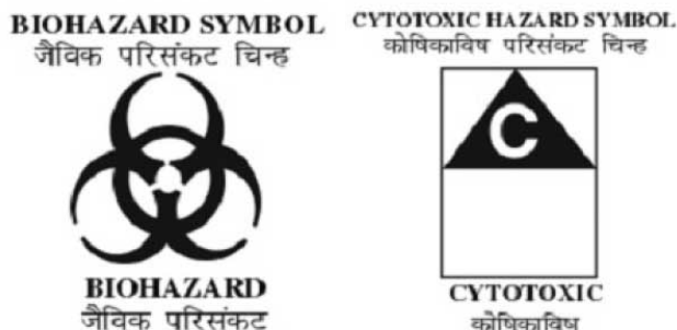
Schedule III: Label for Bio-Medical Waste Containers/Bags
