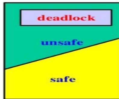
Fig: safe, unsafe, and deadlock state space
