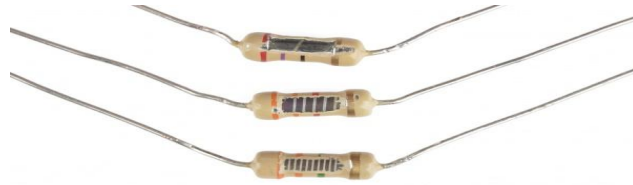
Figure 1.3: Peek inside the guts of a few carbon-film resistors. Inside the resistor, a carbon film is wrapped around an insulator. More wraps means a higher resistance. Pretty neat!
