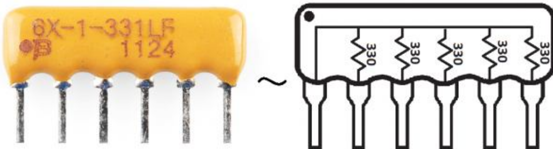
Figure 1.4: An array of five 330\Omega resistors, all tied together at one end.
